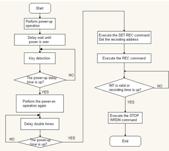
Figure 4: The recording program flow chart diagram
