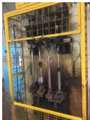
Figure 2: Double-action durability test
