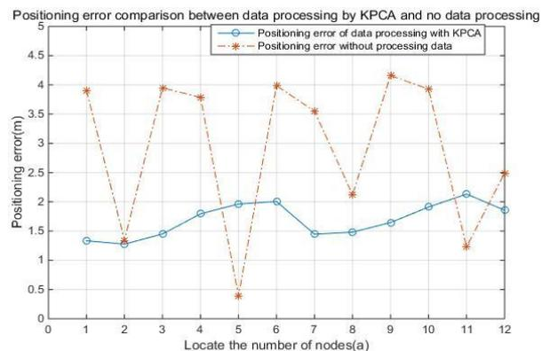
Figure 5: Data preprocessing and no processing error comparison
