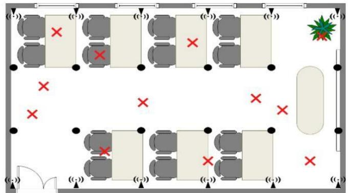
Figure 4: KPCA combined with BP neural network localization results. In the graph,  $\star$  represents the location of the target node,  $\bullet$  represents the coordinate position of the reference node, and  $\times$  represents the positioning result of the KPCA combined with the BP neural network.
