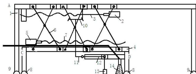
1. supporting frame 2. Motor 3. Screw 4. scrubbing support mechanism 5. Motor 6. folding bracket 7. Screw 8. scrubbing support mechanism sucker 9. support frame with sucker 10. Gear 11. Disc 12. connecting rod and slider 13. Cleaning 14. cleaning liquid nozzle
