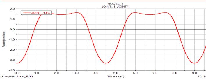
Figure 10: The force between rod and the crank
