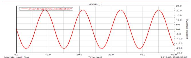
**Figure 9:** Acceleration of fixed point of transmission rod
